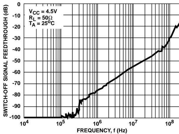
FIGURE 3. TYPICAL SWITCH-OFF SIGNAL FEEDTHROUGH vs FREQUENCY
