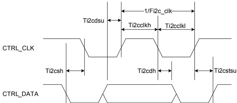
**Figure 5. I<sup>2</sup>C Timing (CTRL\_MODE == 0)**
