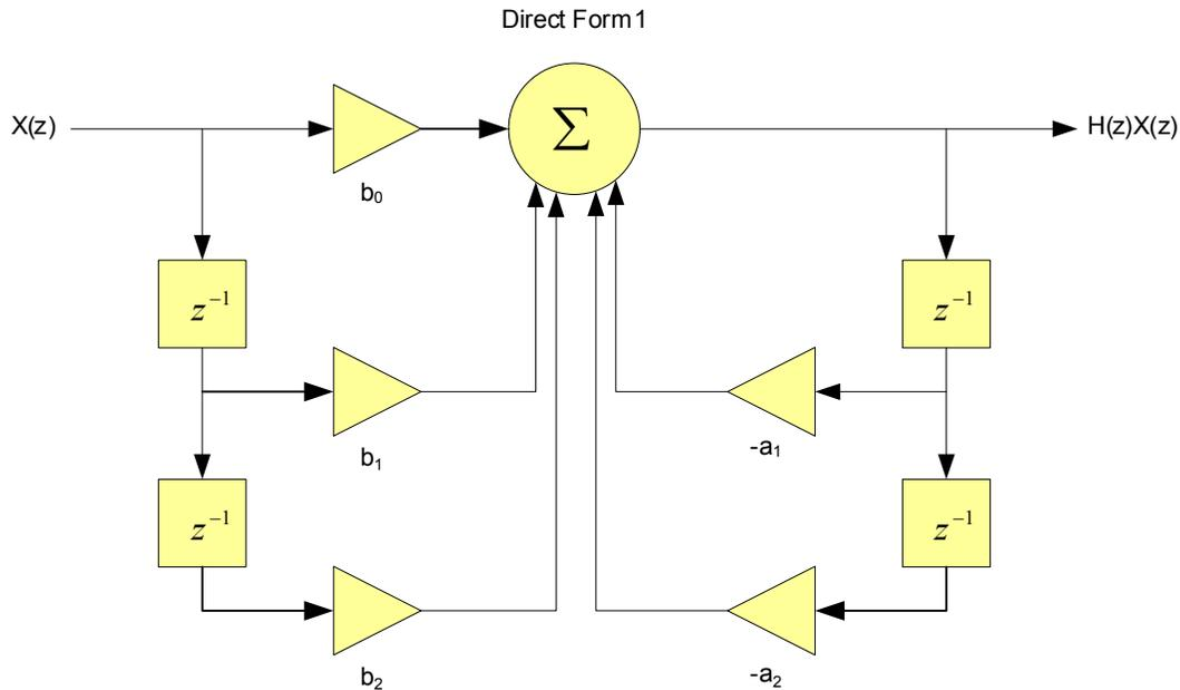
**Figure 15. 5-Coefficient Biquad Filter and Transfer Function**
