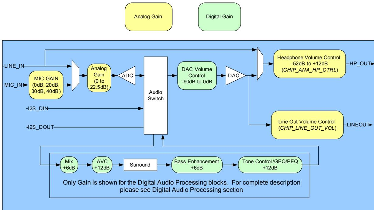
Figure 8. System Block Diagram, Signal Flow and Gain
