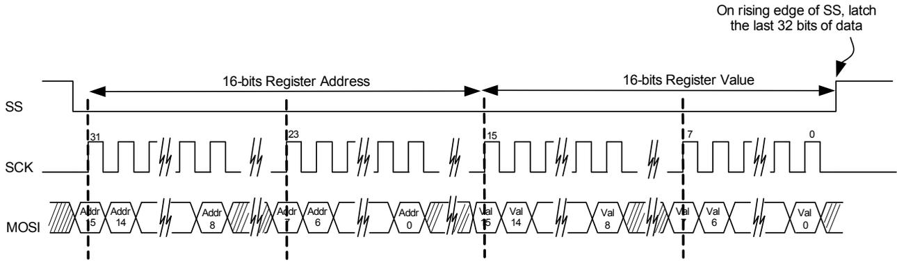
Figure 18. Functional Timing Diagram of SPI Protocol
