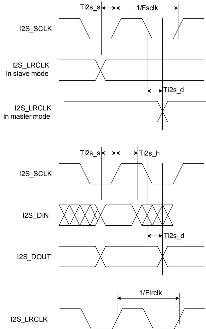
Figure 7. I<sup>2</sup>S Interface Timing
