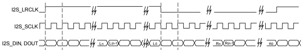
Figure 10. I<sup>2</sup>S Port Supported Formats
