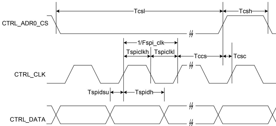
**Figure 6. SPI Timing**
