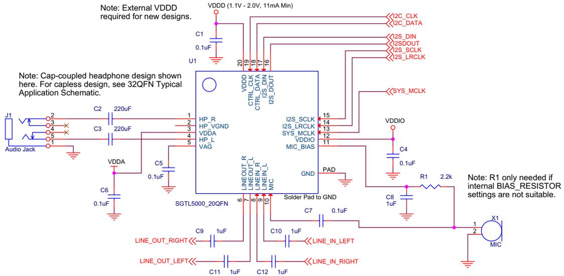
Note: Bottom PAD/FLAG/Paddle MUST be connected to ground.
