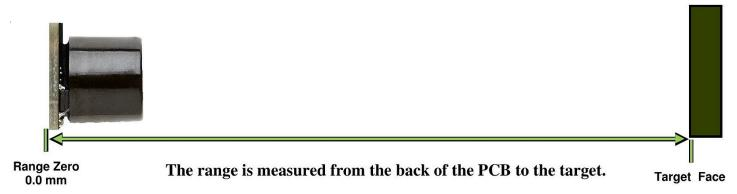
In general, the HRLV-MaxSonar-EZ will report the range to the leading edge of the closest detectable object. Target detection has been characterized in the sensor beam patterns.
