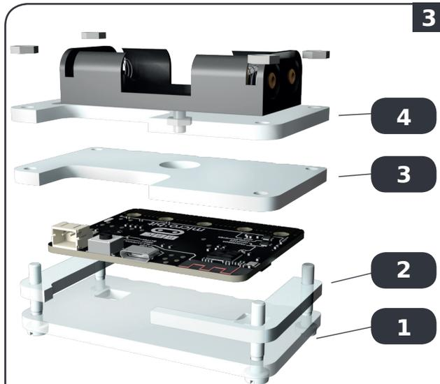
Stack each layer as numbered onto the screws through layer no. 1, then tighten nuts.
